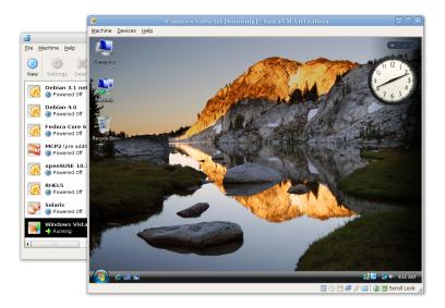
VirtualBox allows the guest code to run unmodified, directly on the host computer, and the guest operating system "thinks" it's running on a real machine. In the back-
